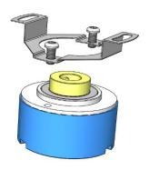
KEM encoder is usually using hollow shaft to allow motor shaft directly inserting into the hollow, it shall be mounted by a flexible mounting plate as shown in figure above. Make sure to fix the shaft in that the mounting plate will not cause burden the ball bearing to the encoder and will not cause damage to the mounting plate.
