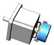
Couple the encoder hollow shaft with the rigid motor shaft and always fasten attached screws securely. Be sure to firmly tighten two hex-screws that located at encoder' s hollow shaft, apply threads-lock glue and tightly screwed in for long-term use.
